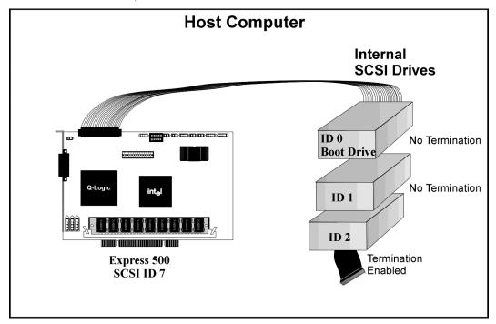
**Terminating External Disk Arrays** In most array enclosures, the end of the SCSI cable has an independent SCSI terminator module that is not part of any SCSI drive. In this way, SCSI termination is not disturbed when any drive is removed, as shown below:
